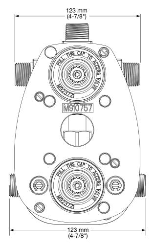
**Solid Brass Inlet Connections:** Fast and easy installation without adaptors reducing leak points - Easier and flameless installation (no soldering required)
