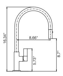
Pull down aerator with dual function spray Swivel spout 1.75 GPM (6.6 L/min.)
