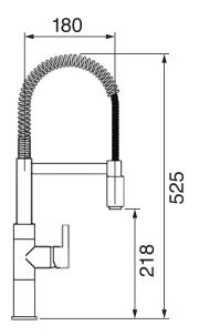
Dual spray Swivel spout 1.75 GPM (6.6 L/min.)
