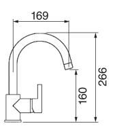
Swivel spout 1.75 GPM (6.6 L/min.)
