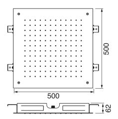
20" x 20" (500 mm x 500 mm) Easy clean nozzles Recessed built in frame High polished stainless steel 2.5 GPM (9.5 L/min.)
