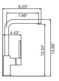
Swivel spout 1.75 GPM (6.6 L/min.)
