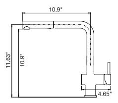
Pull out spout with dual function spray Swivel spout 1.75 GPM (6.6 L/min.)
