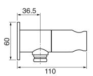
Round metal sprayer with square flange Easy clean nozzles 1/2" male NPT inlet Turn mounting hook for on-off Easy slide installation
