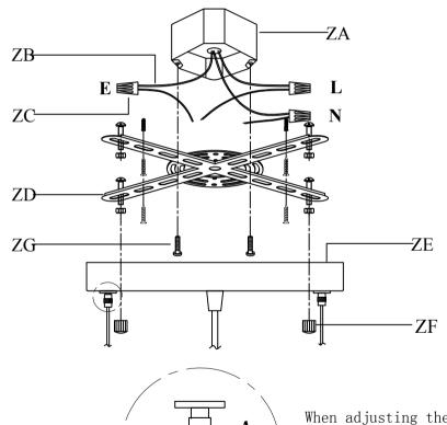
When adjusting the height of the steel wire, the telescopic metal part A toothed outer ring can only twist half a turn, and then pull it up to adjust the height!!!
