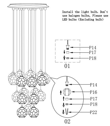
01. Unscrew the lamp holder ring (P18) counterclockwise, and then remove the iron tube (P17);
