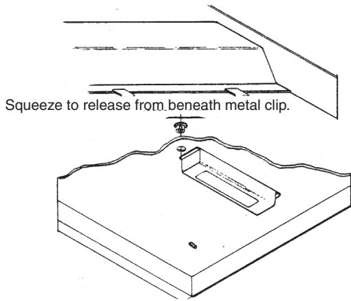
Squeeze to release from beneath metal clip.
