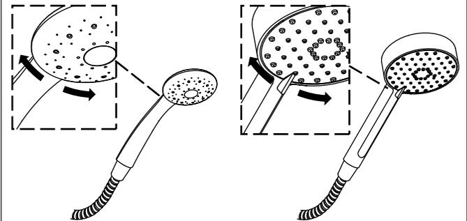
**Maintenance:** To dislodge debris, rub the nozzles or sprayface while the water is running. To improve the water flow, disconnect the handshower and clean the screen washer.
