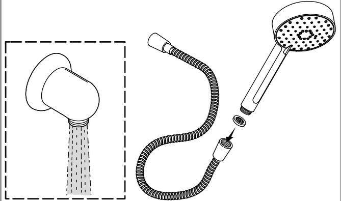
**Operation:** For multifunction handshowers only, rotate the sprayface or use the lever to change the spray options.
