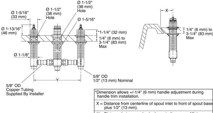
Y = Distance between valve body centerlines vary. Minimum distance is 8" (203 mm).
