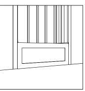
Using a pencil, mark the bathtub flange where the wall studs are.
