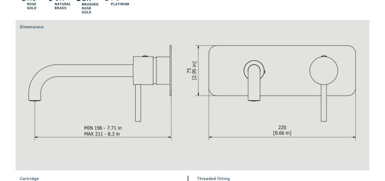
G1/2" female Ø35 ceramic cartridge Aerator Flow Rate (+/-10%) M16.5x1 1 BAR 2 BAR 3 BAR
